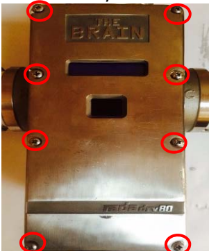
Figure 3: Front Cover Access
